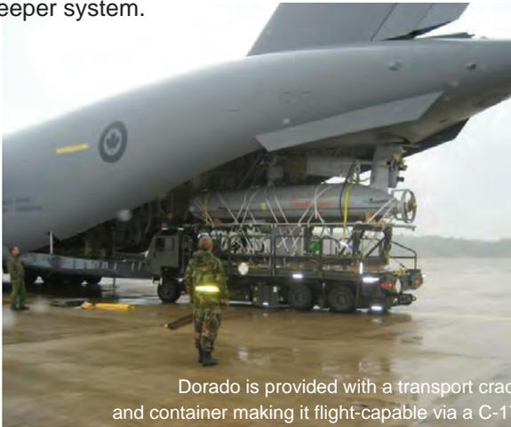
Dorado is provided with a transport cradle and container making it flight-capable via a C-17
