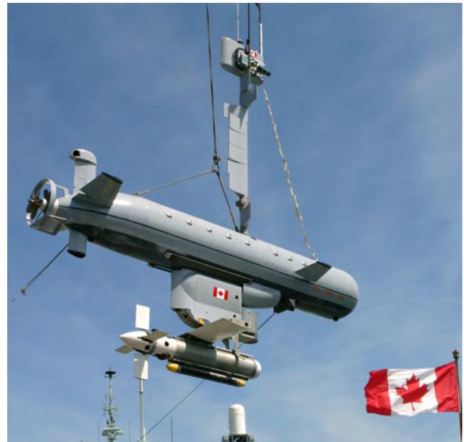
Dorado has a surface-piercing mast, allowing it to operate and transmit sonar data over a radio data link
