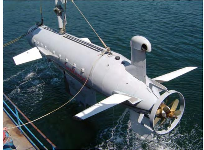
The Dorado vehicle is capable of towing a sonar towfish at speeds up to 12 knots and depths to 200 m. It is powered by a 315 kW marine diesel engine. Air is drawn through the mast and exhausted through the stabilizer above the contra-rotating propeller. The engine also provides power for the hydraulically operated control planes and the keel-mounted winch for the sonar towfish. The towfish is developed to follow the seabed at low altitudes and is fitted with a multibeam sidescan sonar.
